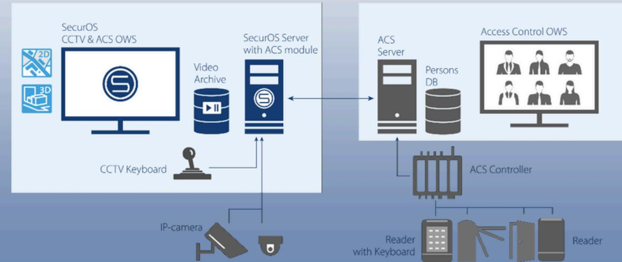
SecurOS GUI Operator Workstation (OWS) is expanded with the ACS / Fire alarms operator's functionality
