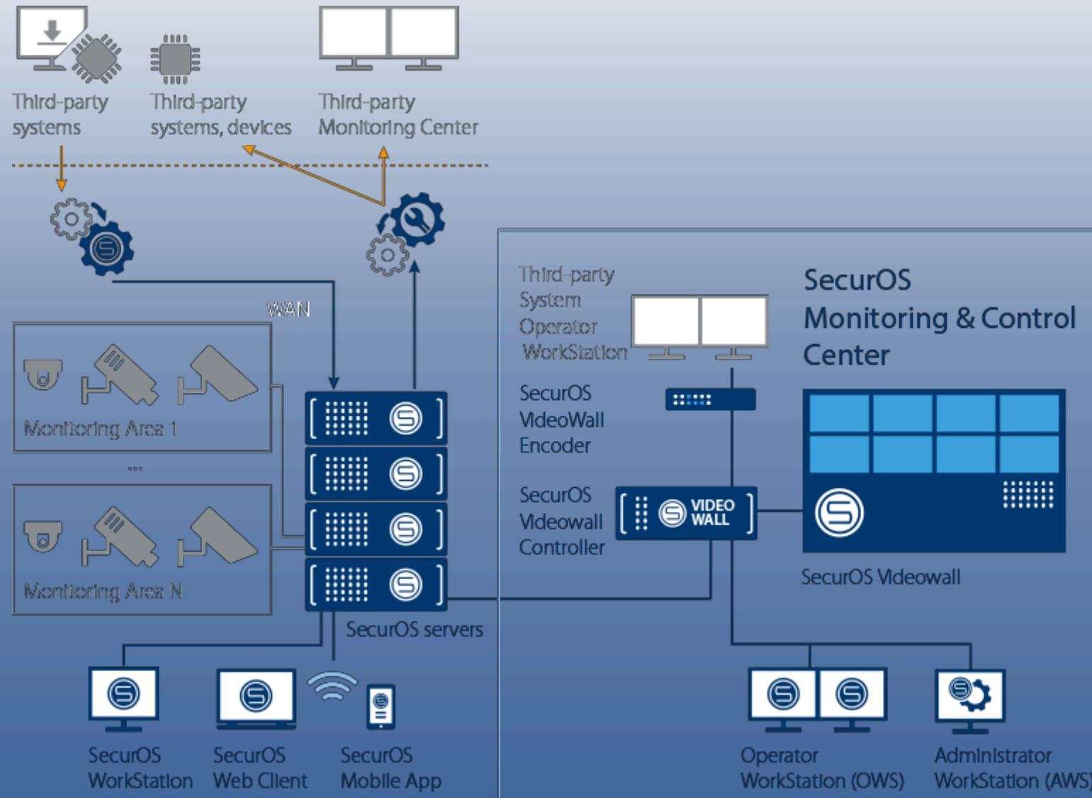
SecurOS integrates a multitude of IS and third party systems into one integrated network and creates a unified command and control capability.
